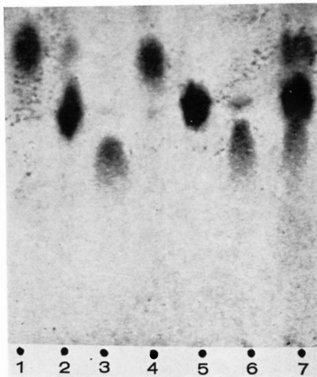
FIG. 2. Silicic acid-impregnated glass paper chromatography of 1, peak III; 2, peak IV; and 3, peak V compared to the standards 4, lecithin; 5, sphingomyelin; 6, lysolecithin; and 7, a mixture of the three standards. The spots represent 20 \mu\text{g} of phospholipid from the complete pooled peaks derived from four column fractionations. This amount of phospholipid represents an overload in order to detect small quantities of impurities. As little as 0.1 \mu\text{g} phospholipid is detectable by the charring technique. The top of the photograph represents the solvent front. The solvent mixture was phenol-diethyl ether-acetone-water.
